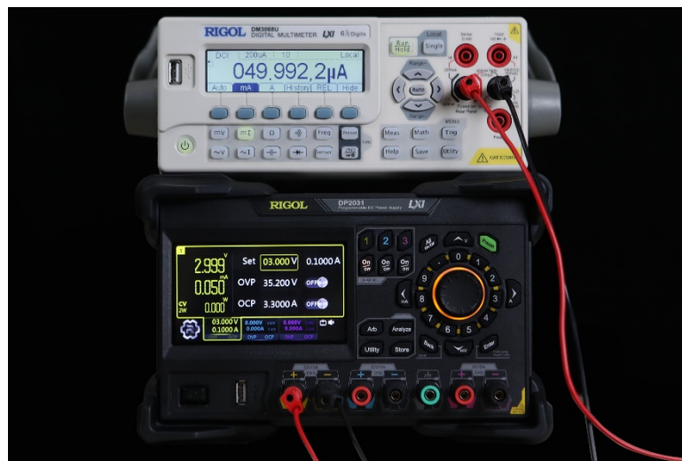
Figure 4.10 DP2000 Provides uA-level Precision Current
