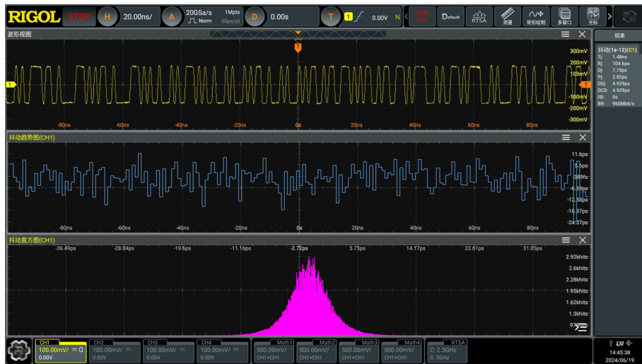
Figure 5.2 LVDS Signal Jitter Test Results
