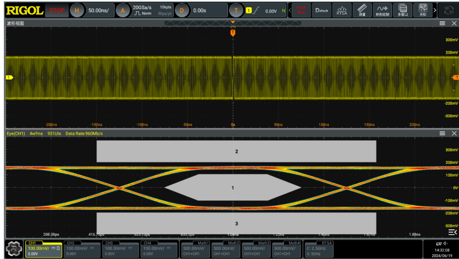
Figure 5.1 LVDS Eye Diagram Test Results
