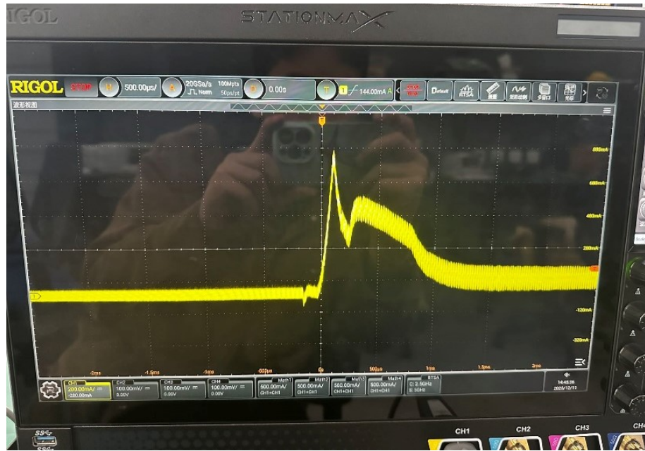
Figure 5.3 Tests Result for Rush Current at Power-up Moment
