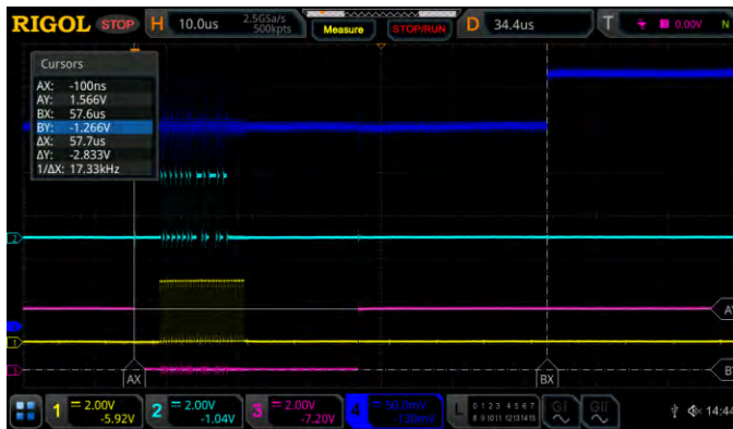
Figure 4: Latency measurement from SPI bus to LED on our IoT development board
