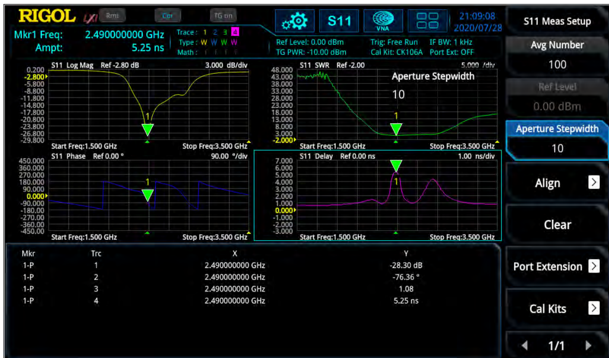
Figure 7: S 11 measurement: logarithmic magnitude of |r|; phase over-, SWR over- and group delay over frequency
