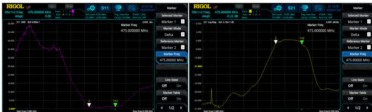
Figure 8: left side: S 11 SWR measurement; right side: S 21 insertion loss (logarithmic magnitude) measurement
